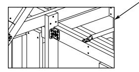
Use brackets as a drill guide and drill 1/8" holes 1" deep into the boards. Attach with #8 x 11/4" deck screws.
