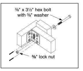
Securing through <u>two</u> boards use %" x 3½" hex bolt.
