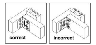
Caution: If the bracket was flipped and the short side was against the double board when you drilled, the holes will be too close to the edge of the vertical 2" x 4".
