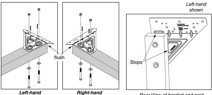
Rear View of bracket and post assembly showing correct position.
