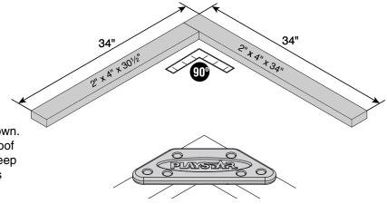
On a flat surface position boards together as shown. Position roof cap flush with outside edges. Use roof cap as a drill guide and drill  $\frac{1}{8}$  holes 1" deep. Keep boards square while attaching roof cap to boards with #14 x 1 $\frac{1}{4}$ " pan head screws.
