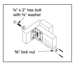
Securing through <u>one</u> board use <sup>3</sup>/<sub>8</sub>" x 2" hex bolt.
