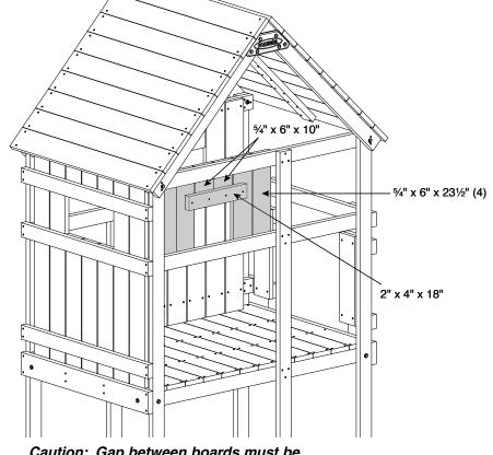
Caution: Gap between boards must be smaller than ¼" or larger than ½" or a finger entrapment could exist.
